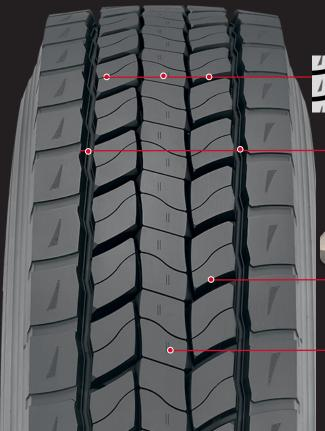
Lateral support between blocks helps maintain the tread's ideal shape for enhanced road contact and grip.
