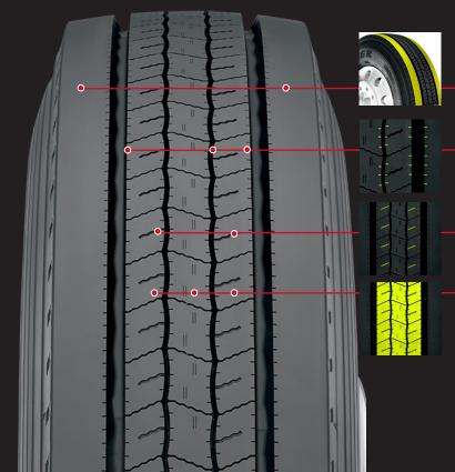
Resist tearing and provide uniform surface pressure to resist irregular wear.
